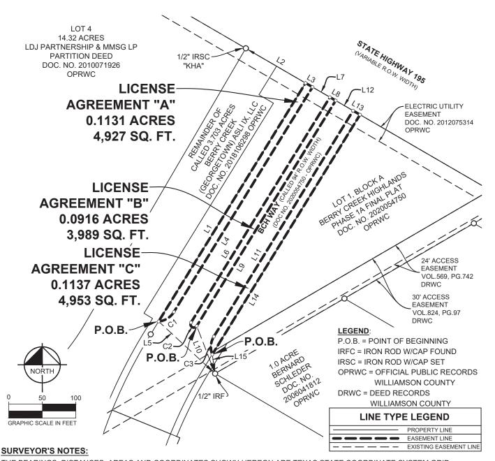
THE BEARINGS, DISTANCES, AREAS AND COORDINATES SHOWN HEREON ARE TEXAS STATE COORDINATE SYSTEM GRID, CENTRAL ZONE (FIPS 4203) (NAD'83), AS DETERMINED BY THE GLOBAL POSITIONING SYSTEM (GPS). THE UNIT OF LINEAR MEASUREMENT IS U.S. SURVEY FEET. A METES & BOUNDS DESCRIPTION AND A LINE & CURVE TABLE WAS CREATED IN CONJUNCTION WITH THIS LICENSE AGREEMENT EXHIBIT.
